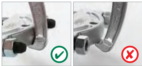
Firmly affix bearing separator and align legs
