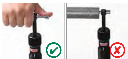
Hand operation only should be used to achieve force
