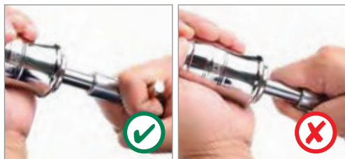
Keep hands away from contact area while slide hammer is in use
