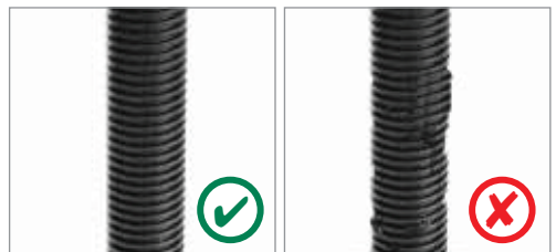
Frequently lubricate and inspect forcing screw for damage
